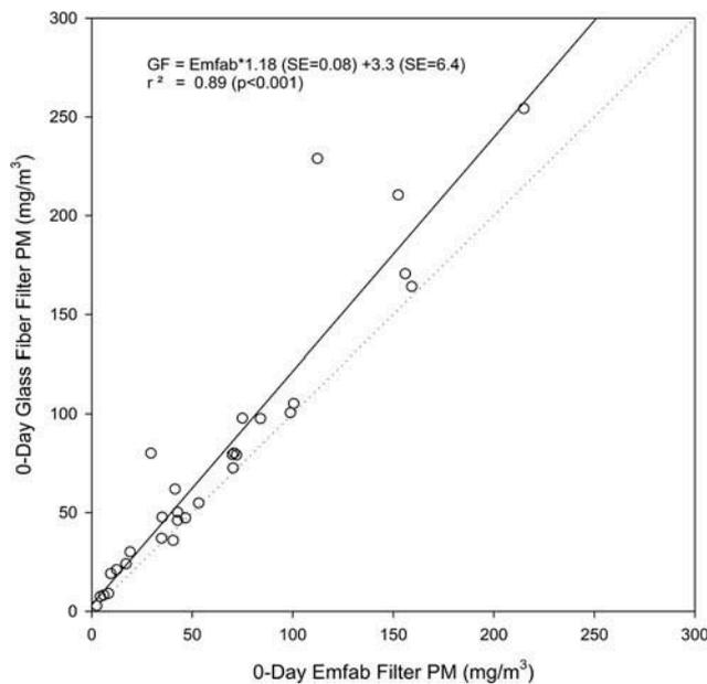
**Figure 1.** 0-Day glass fiber filter versus 0-day Emfab filter PM concentration (mg/m<sup>3</sup>).
