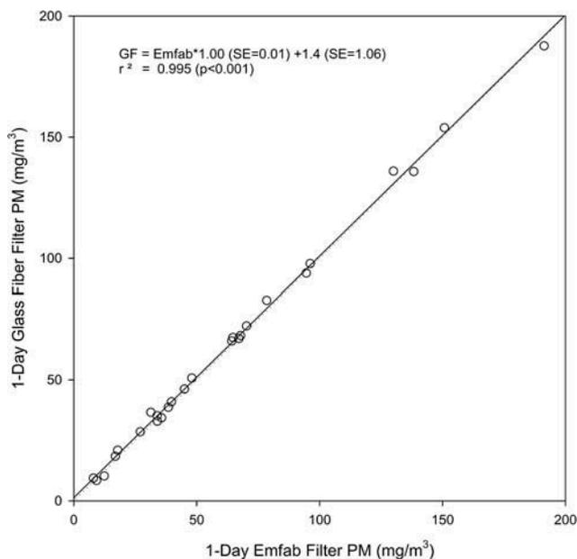
**Figure 3.** 1-Day glass fiber filter PM concentration versus 1-day Emfab filter PM concentration ( $\text{mg}/\text{m}^3$ ).
