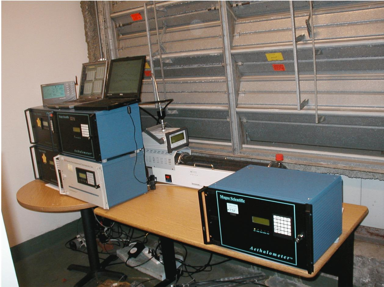
Left to right: weather console, four Aethalometers, DR-4 nephelometer, thermodenuder, thermodenuded Aethalometer.
