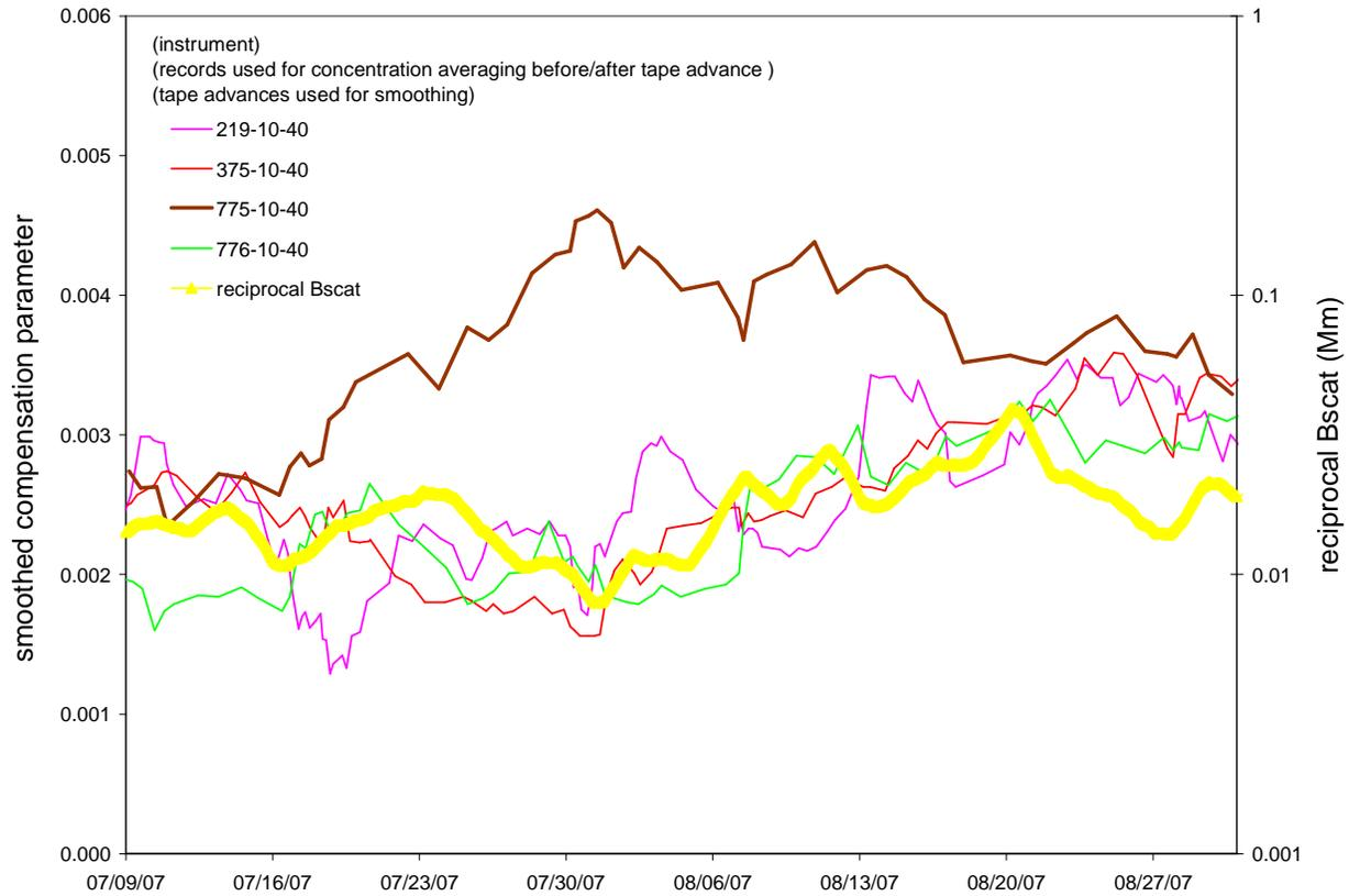
In this figure, the brown line is the K factor from the thermodenuded Aethalometer. It has a higher K factor, indicating a more sooty (winter-like) aerosol. The thick yellow line is the inverse of the scattering data, plotted on a log scale. The K factor for the non-denuded Aethalometers roughly follows this line as expected, since an aerosol with higher scattering would produce less spot saturation and thus a lower K factor.
