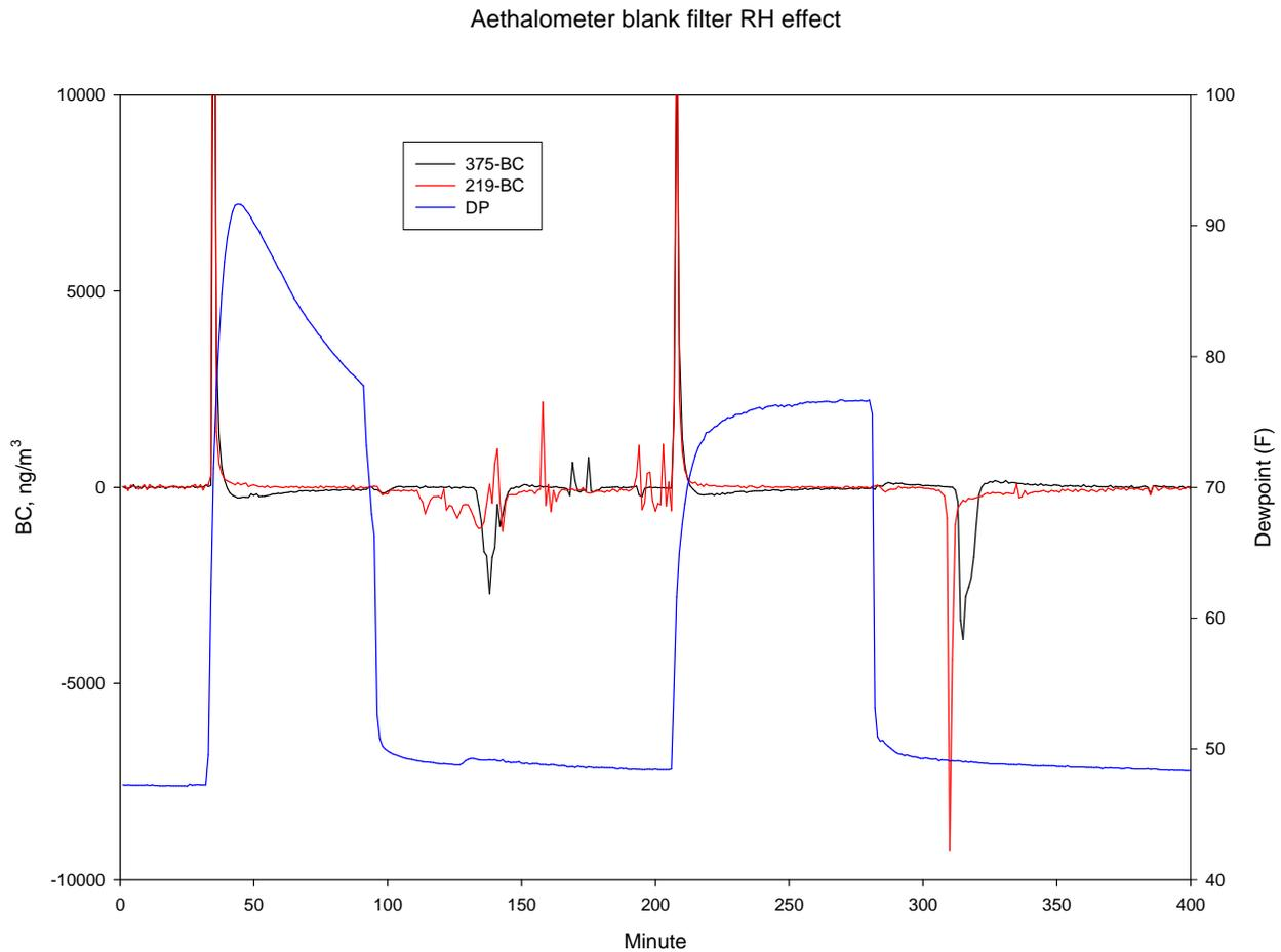
In this work, the short-term (1-minute) noise from both the Aethalometer with the Nafion drier and the thermodenuded Aethalometer was substantially lower than “normal” Aethalometers. A simple metric of short-term noise is the standard deviation of the difference between subsequent 1-minute BC data points. For the post-test period Sept. 21-Oct. 8 and using normalized data to remove between instrument bias, this sigma in  $\mu\text{g}/\text{m}^3$  is as follows:
