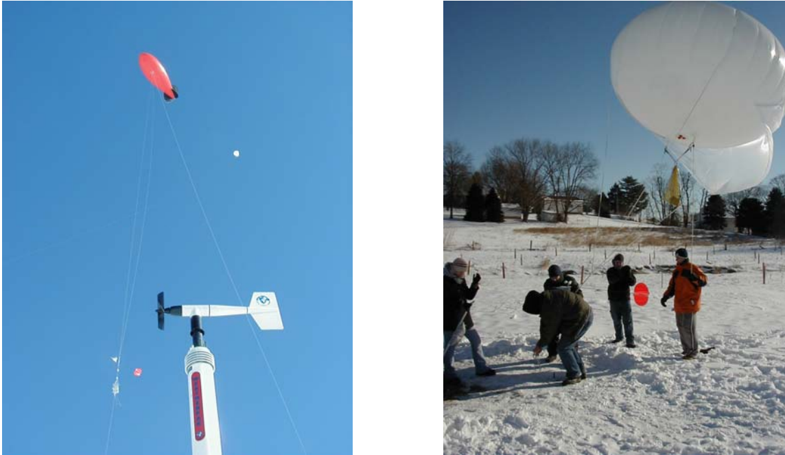
Fig. 1. Left: Blimp used for vertical profiling (BP); Right: Balloon used for constant altitude time series (CA).
