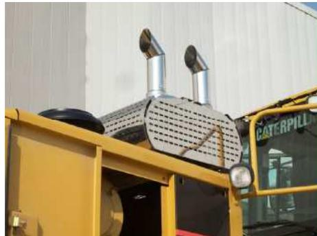
**Figure 2:** 988H loader retrofitted with dual DPFs, showing shield in place
