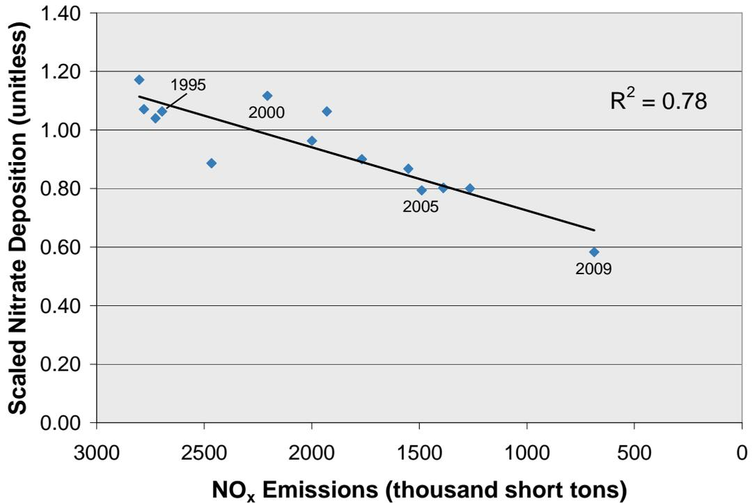
Figure Caption: Annual fossil fuel power plant NO<sub>x</sub> emissions correlation with the combined nitrate precipitation-weighted and total wet deposition scaled to a mean of unity in the New England region from 1995 to 2009. Points are labeled at ~5-year intervals to help illustrate trend over time. Note that emissions on x-axis are plotted on a decreasing scale from left to right.
