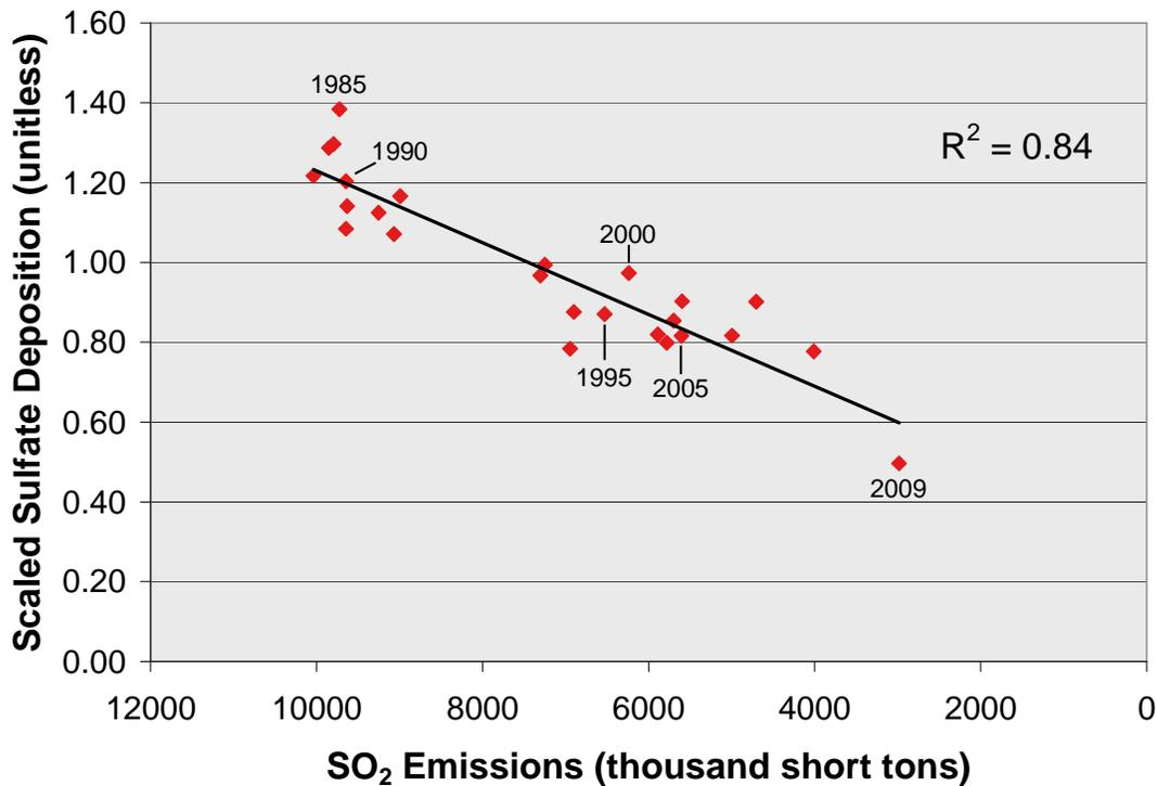
Figure caption: Annual fossil fuel power plant sulfur dioxide (SO<sub>2</sub>) emissions correlation with the combined sulfate precipitation-weighted and total wet deposition scaled to a mean of unity in the New England region from 1985 to 2009. Points are labeled at ~5-year intervals to help illustrate trend over time. Note that emissions on x-axis are plotted on a decreasing scale from left to right.
