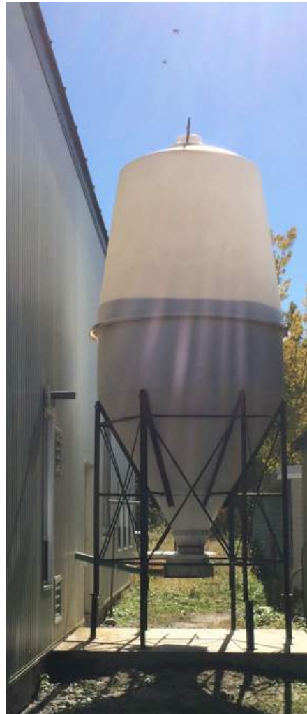
Polydome silo (8.5 ton capacity)
