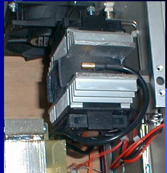
Cooled preconcentration trap
