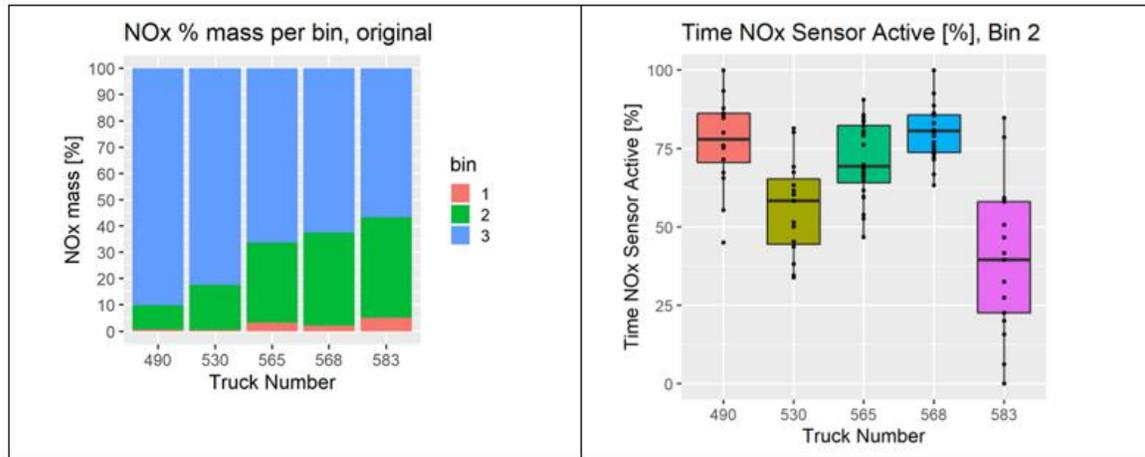
Figure 6: NOx mass in bins 1, 2, and 3 (left); and time NOx sensors were active in bin 2 for each of five trucks data logged (right).
