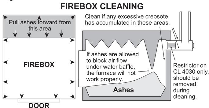
Clean corners as indicated by arrows in illustration. Pull ashes forward from the back of the firebox in shaded area. The walls of the firebox should be scraped from the ash line and below. Clean excessive creosote as necessary.
