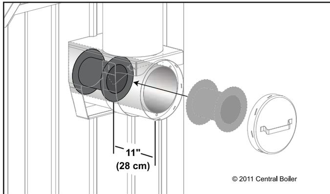
3. **Check for leaks.** Close the valves on the outdoor furnace before checking for leaks. Do not pressurize the outdoor furnace. Pressure-test the entire plumbing system. Apply 50 psi (3.5 kg/cm<sup>2</sup>) of air pressure for thirty minutes and closely monitor for any pressure loss. Inspect all fittings and hose ends for any signs of leakage using leak detection solution (leak soap); repair as necessary.
