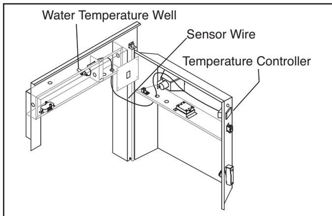
To test the water temperature sensor using a multimeter, see Testing Water Temperature Sensor. If the sensor needs to be replaced, see Replacing Water Temperature Sensor.
