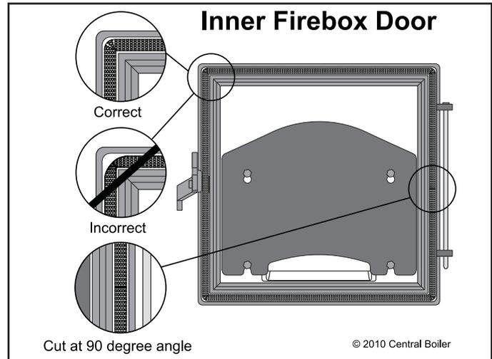
6. When the seal has been pressed into the groove all the way around the firebox door, cut the end of the rope about one inch (2,5 cm) longer than required and press it tightly against the beginning end of the rope.
